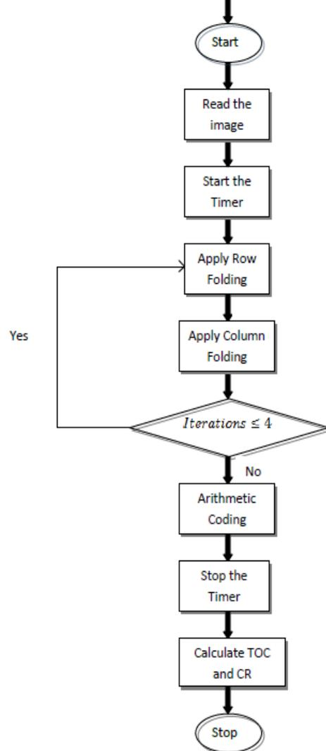
Fig.4 Flow Chart for Compression Procedure
