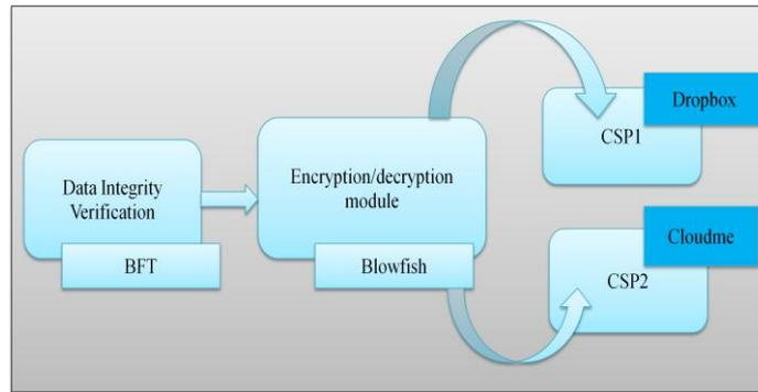
Figure 3: Workflow of a proposed architecture
