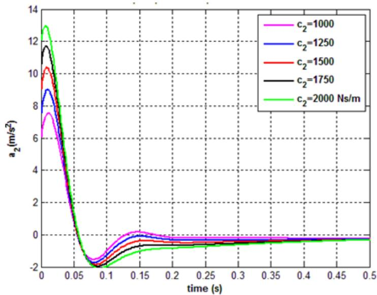
Fig.11 Sprung-mass step response (acceleration) for  $k_2 = 2000$  N/m.
