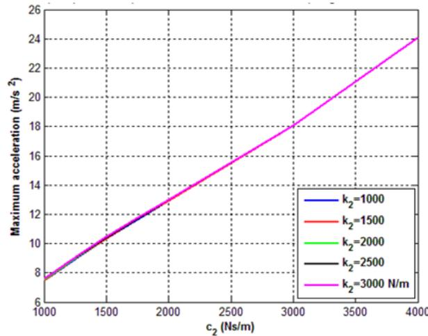
**Fig.14** Maximum acceleration of the sprung-mass due to the step input.
