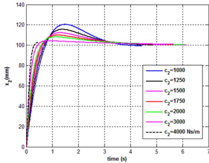
Fig.2 Sprung-mass step response for  $k_2 = 1000$  N/m.
