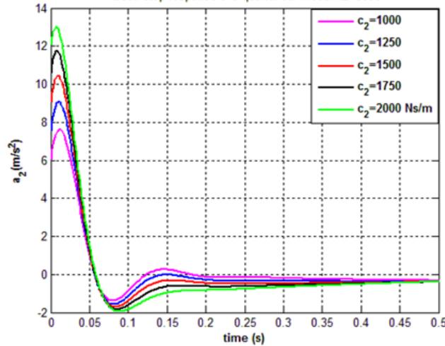
**Fig.13** Sprung-mass step response (acceleration) for  $k_2 = 3000$  N/m.
