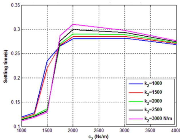
**Fig.15** Settling time of the sprung-mass due to the step input.
