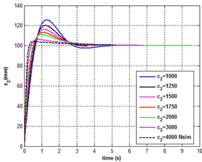
Fig.3 Sprung-mass step response for  $k_2 = 1500$  N/m.
