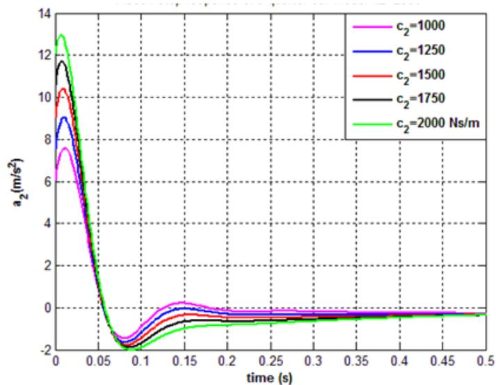
Fig.12 Sprung-mass step response (acceleration) for  $k_2 = 2500$  N/m.
