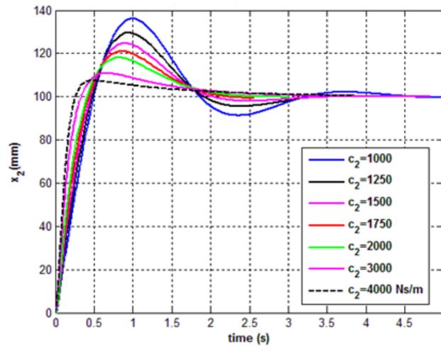
Fig.6 Sprung-mass step response for  $k_2 = 3000$  N/m.
