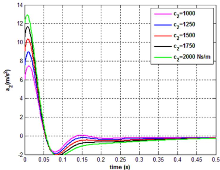
Fig.9 Sprung-mass step response (acceleration) for  $k_2 = 1000$  N/m.
