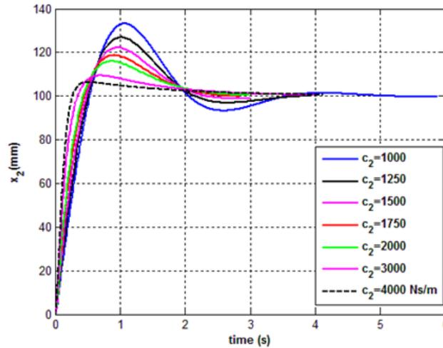
Fig.5 Sprung-mass step response for  $k_2 = 2500$  N/m.
