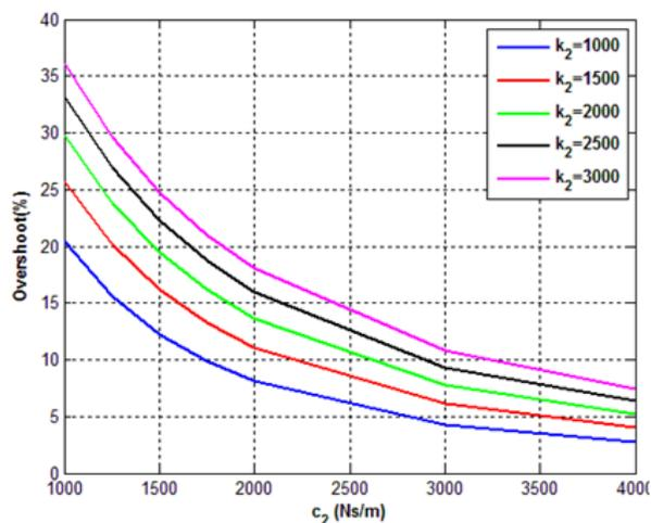
Fig.7 Sprung-mass maximum displacement overshoot.
