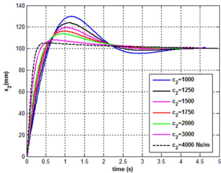
Fig.4 Sprung-mass step response for  $k_2 = 2000$  N/m.
