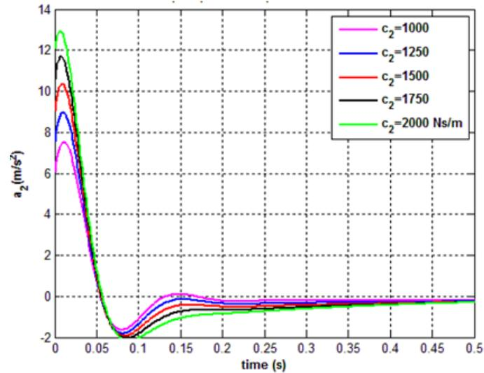
Fig.10 Sprung-mass step response (acceleration) for  $k_2 = 1500$  N/m.
