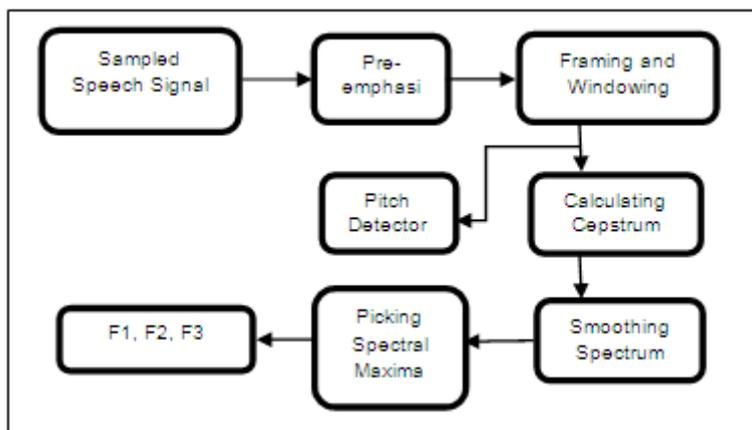
Fig.2. Formant Frequency Estimation Using Cepstral Analysis
