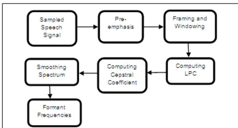
Fig.3. Formant Frequency Estimation Using LPC Analysis
