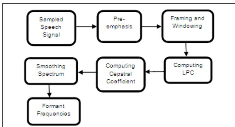
Fig.3. Formant Frequency Estimation Using LPC Analysis
