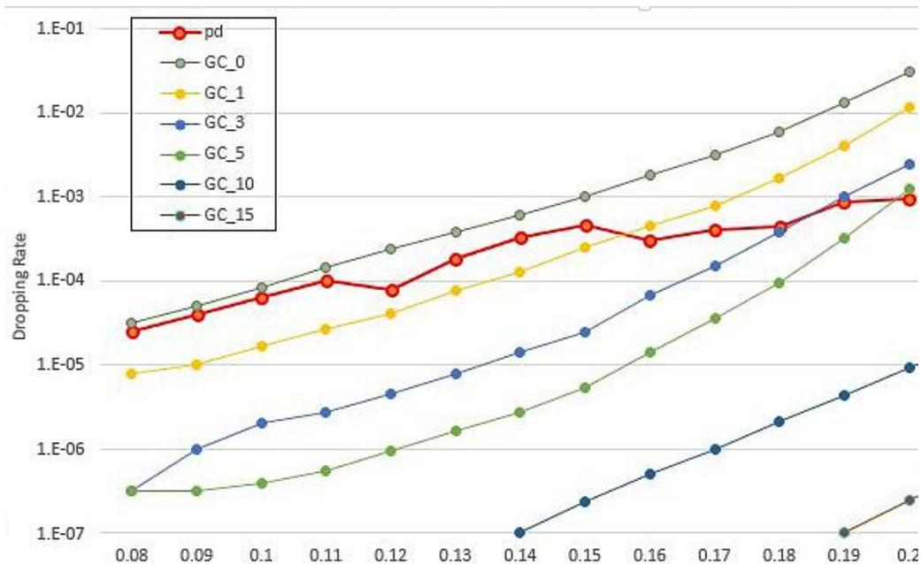
Fig. 4. The dropping rate with different arrival rate of handoff call ( $\lambda_n = 1/6$ ).
