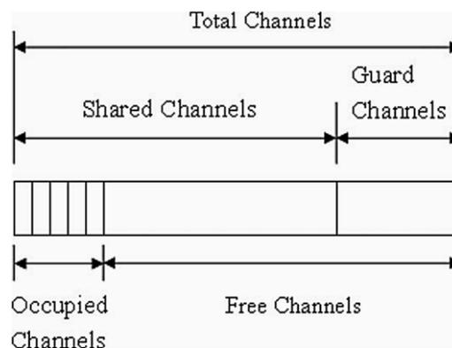
Fig. 1. Guard channel (GC) method.
