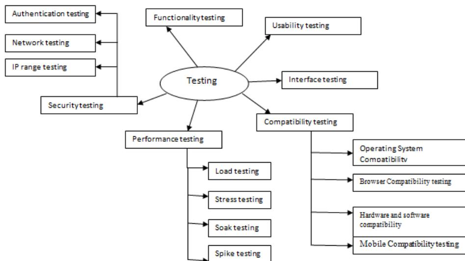
Figure 4. Testing in web application.
