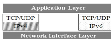
Fig. 1. The Dual Stack Architecture.
