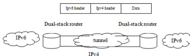
Fig. 2. The IPv6 over an IPv4 Tunnel Architecture
