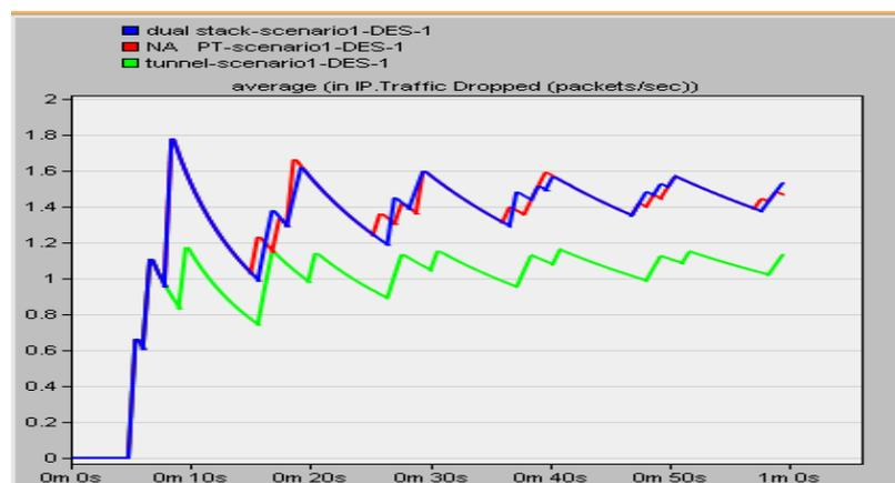
Fig. 6 packet drop (packet loss) for the dual-stack, tunneling and NAT-PT techniques.
