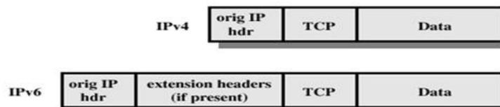
Figure 3: Ipv4 and Ipv6 Datagram without AH
