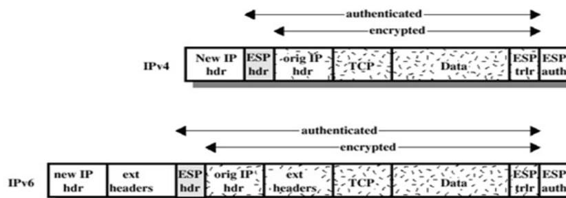
Figure 4: ESP Encryption and Authentication
