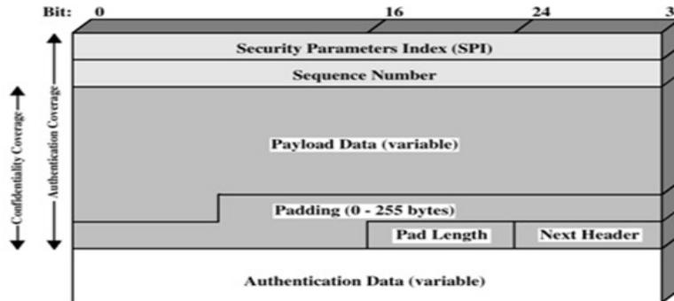
Figure 5: Encapsulating Security Payload
