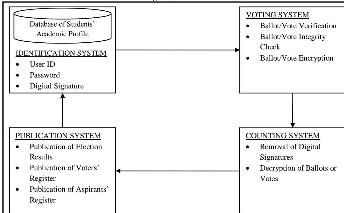
**Figure 2:** Simplified System Architecture of the Secure Intranet Voting System (SIVS)
