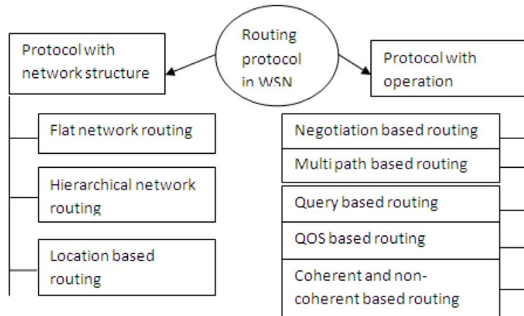
**Figure: 1** Types of routing protocol in wireless sensor network
