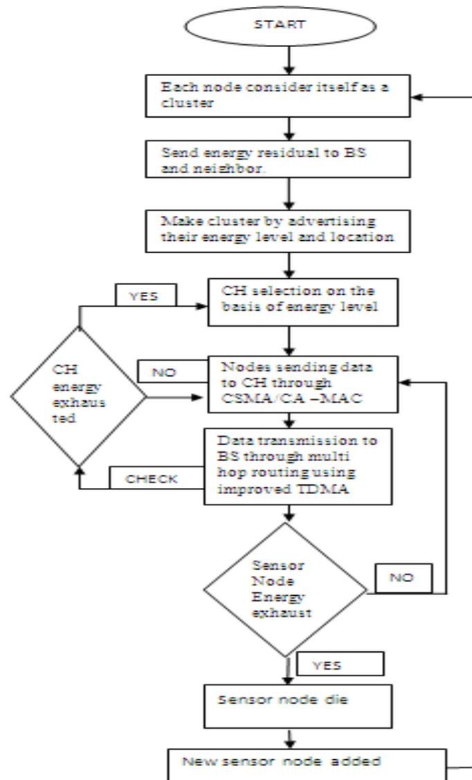
Figure 3. Flow chart for cluster formation and data transmission
