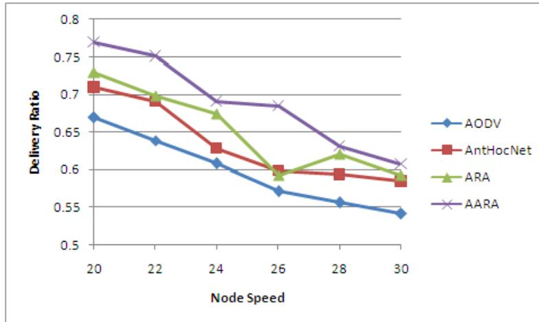
Figure 7.7: Delivery Ratio Vs Node Speed.
