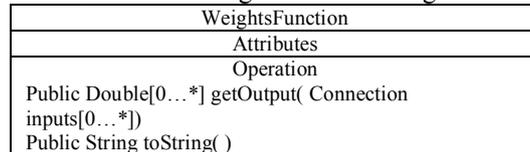
Fig 10. UML Class Diagram for the WeightFunction
