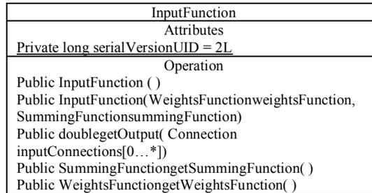
Fig 7.UML Class Diagram for the InputFunction.
