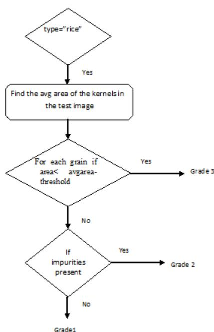
Fig 3.10. Flow diagram for the analysis of rice
