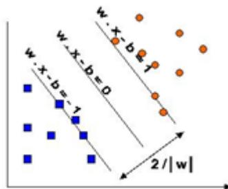
**Fig 3.1.3** Maximum margin hyperplanes for a SVM trained with samples from two classes
