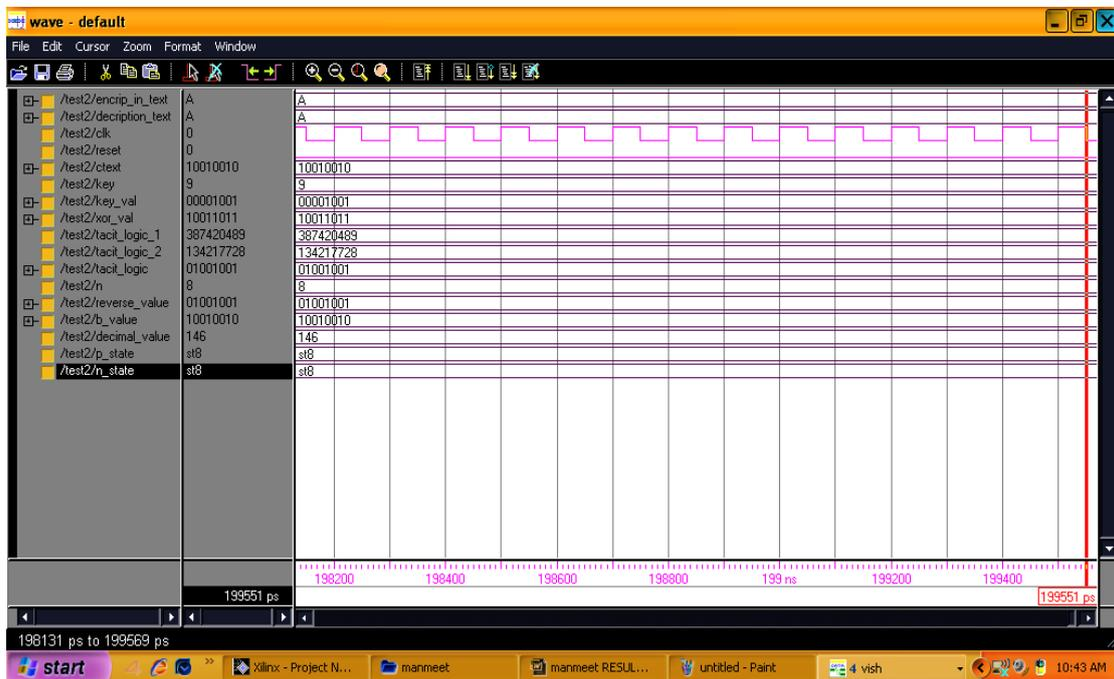
Fig. 6 Modelsim output waveform of decryption (8 bits)
