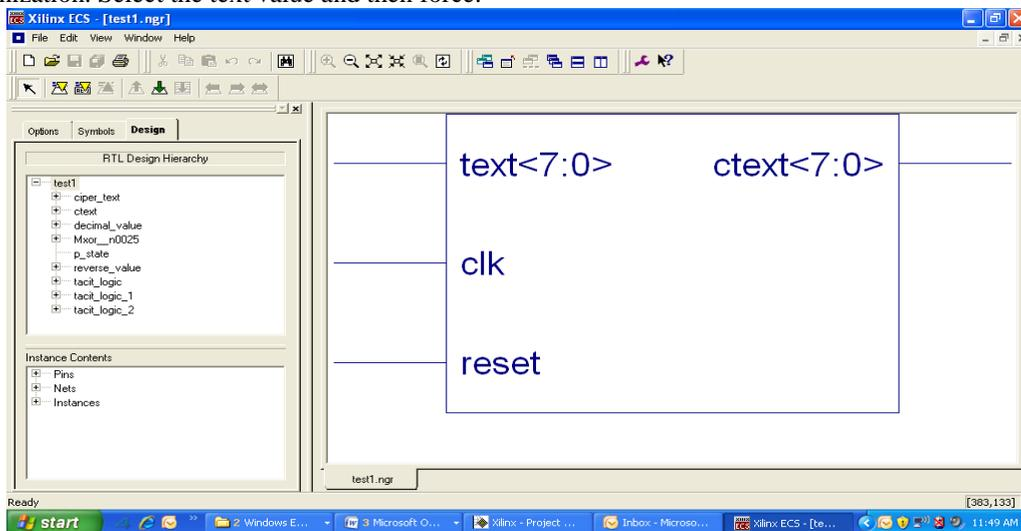
Fig. 3 RTL view of encryption (8 bits data)
