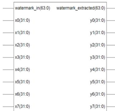
Fig.2 RTL View of DCT with Watermark Chip
