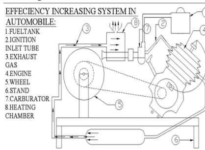
**Fig 2.2 Layout of preheater setup**
