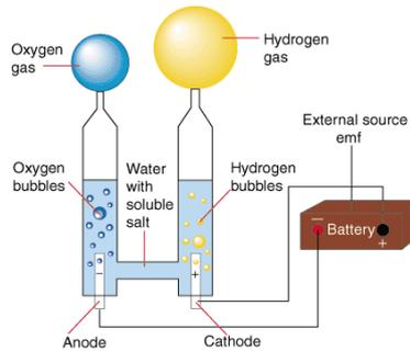
**Fig 1.2 Electrolysis Process**
