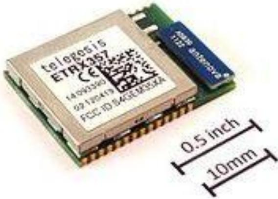
Fig 1: Zigbee Module
