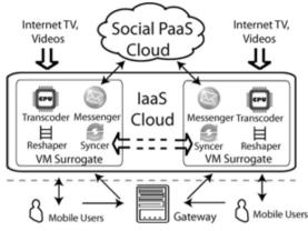
Fig. 1. The architecture of CloudMoV.
