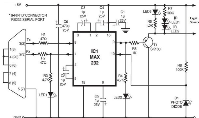
Fig.2: Circuit Diagram for driving LED and photo-diode
