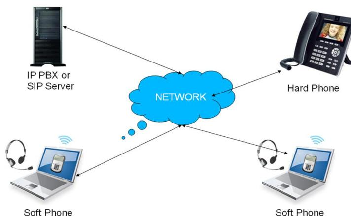
Fig 1 Soft phone Block Diagram
