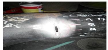
Figure 1:A pipeline showing Crack with measurement (picture courtesy-SADARA,KSA)
