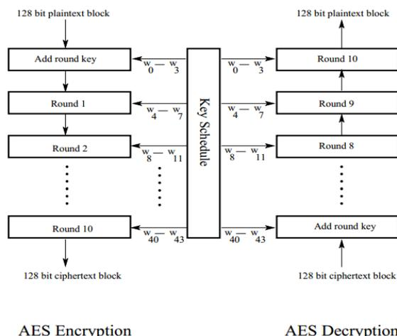
Fig. 5. AES Block Diagram
