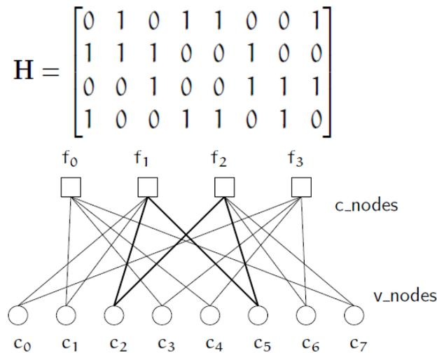
Fig 1. Tanner graph corresponding to the parity check matrix in H. The marked path  $c_2 \rightarrow f_1 \rightarrow c_5 \rightarrow f_2 \rightarrow c_2$  is an example for a short cycle. Those should usually be avoided since they are bad for decoding performance.
