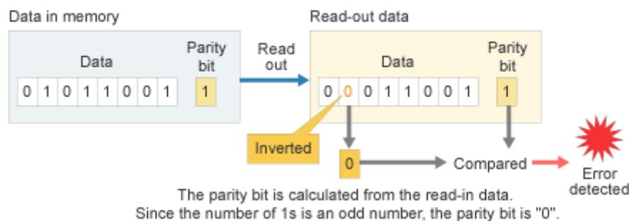
Fig. 5 Error correcting method
