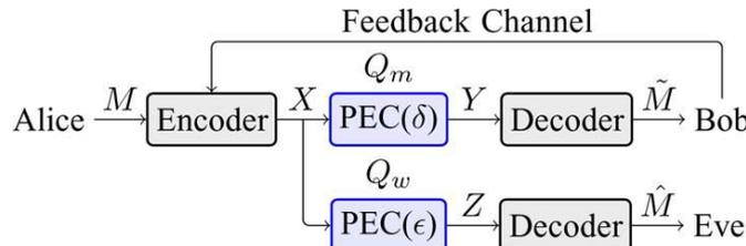
Fig 2. Wiretap channel model with feedback with PECs for both the main channel  $Q_m$  and the wiretap channel  $Q_w$ .
