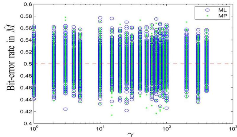
Fig. 6 Simulated bit-error rates in Eve’s decoded cryptogram  $\hat{M}$  when errors are made in guessing bit values for degrees of freedom in Eve’s received codewords.
