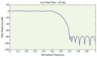
**Figure 1:** A typical low-pass filter maintains low-frequency elements and reduces or removes high-frequency elements in an image.
