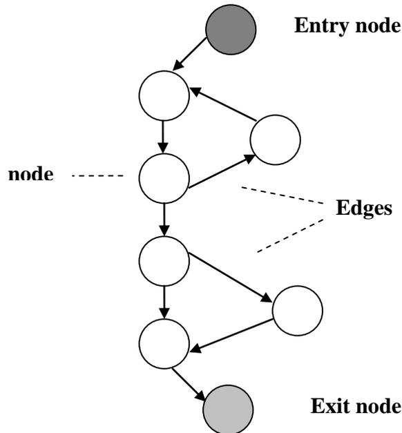
Figure (2): Control flow graph of a simple program [7].
