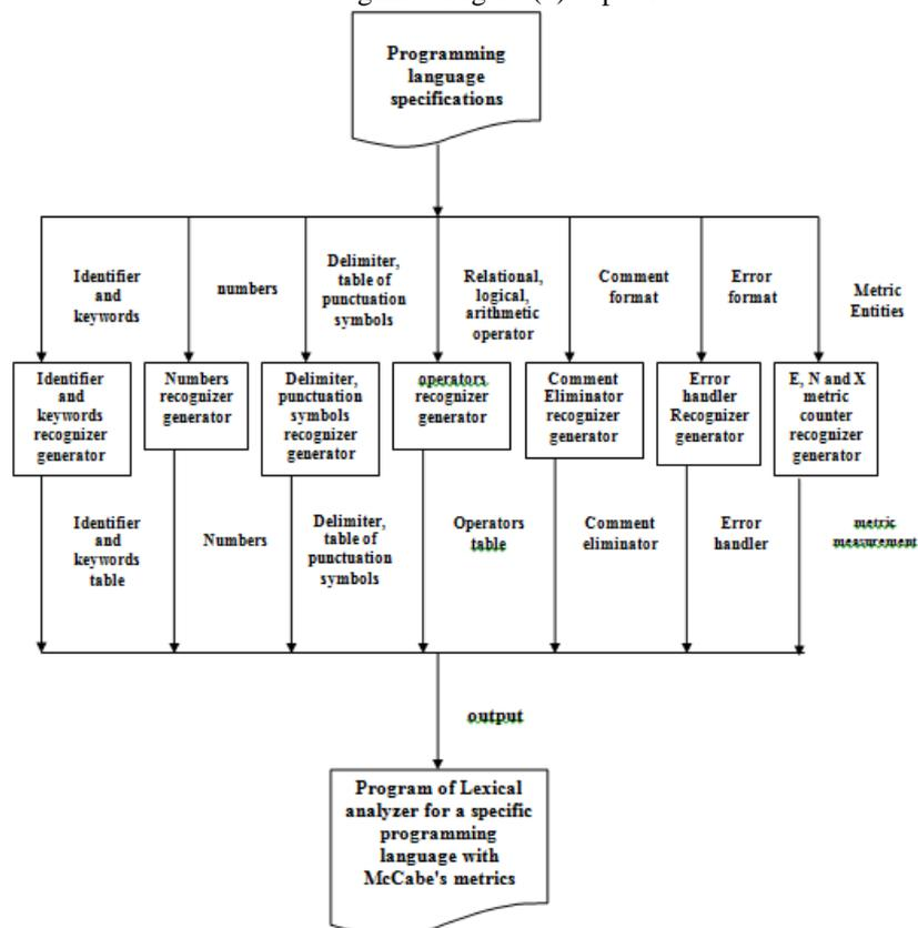
Therefore, LEXIMET consists of many programming parts called, recognizer generators, each of these generators recognizes a specific part of the programming language specification and with a new feature which measures the metrics of any programming language by the E, N, and X counter recognizer to produce a specialized recognizer to be added to the generated lexical analyzer. These generators construct the recognizer as functions. Some of the recognizer generators are:
