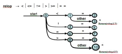
Figure (7): The transition diagram to identify tokens (relational, arithmetic and logical operations ) for C++ language.
