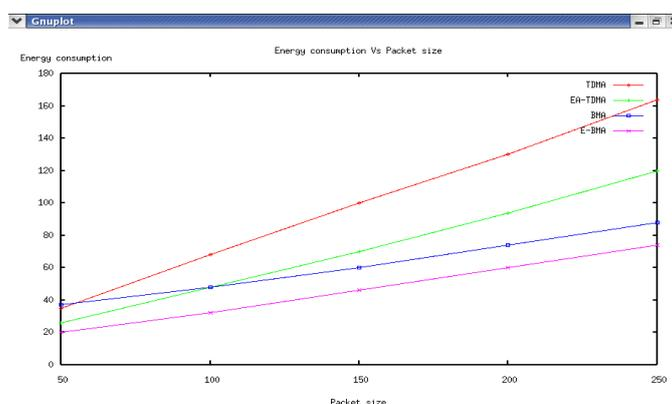
Figure 5.2: Energy consumption with packet size
