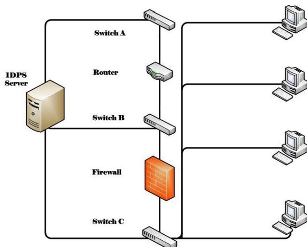
Fig 3. IDPS deployment in a network environment [10], [11].
