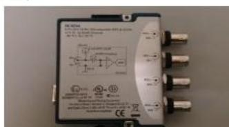
Figure 3: NI-9234 DAQ Board
