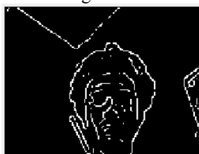
Figure 8: Applying thresholding after the new Edge Detection algorithm to discard the weak edges
