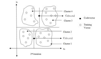
Fig. 4 2<sup>nd</sup> iteration of KFCG Clustering
