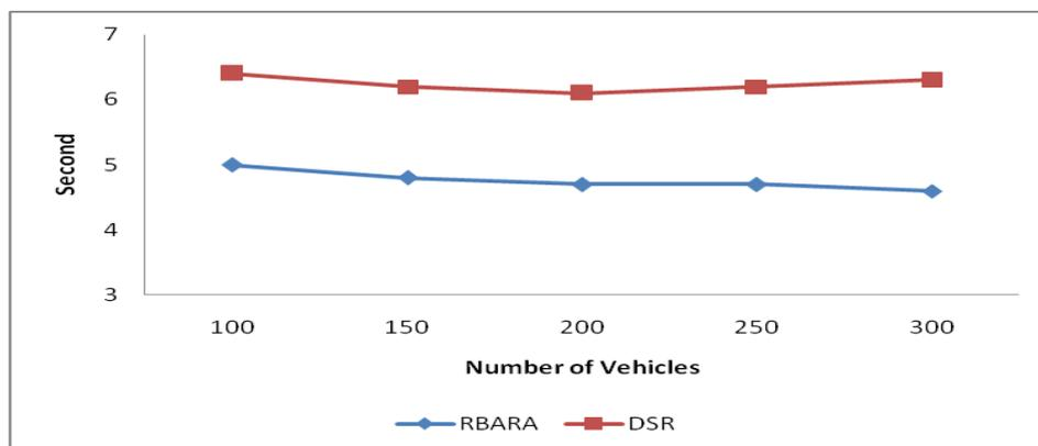
Figure. 7. Transmission Time Dynamic Source Routing vs. Road Based Routing Algorithm
