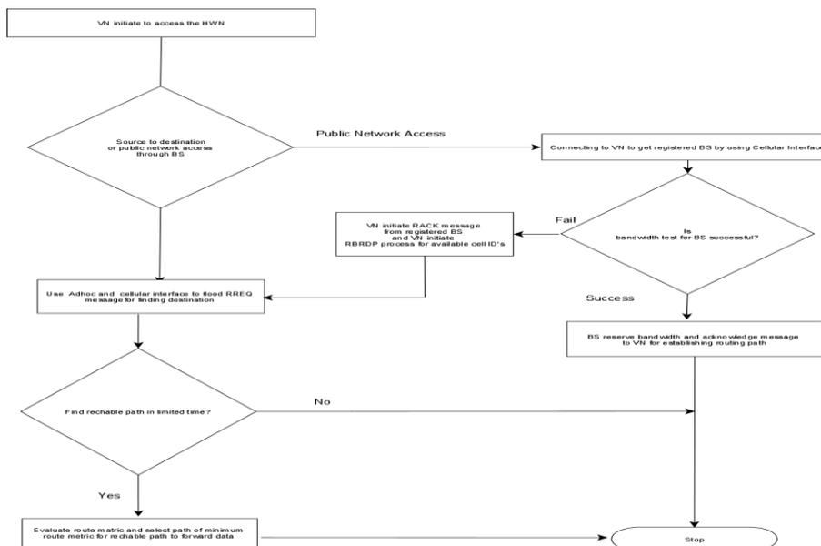
Fig.3. Flowchart Road Based Routing Algorithm in Heterogeneous Wireless Network
