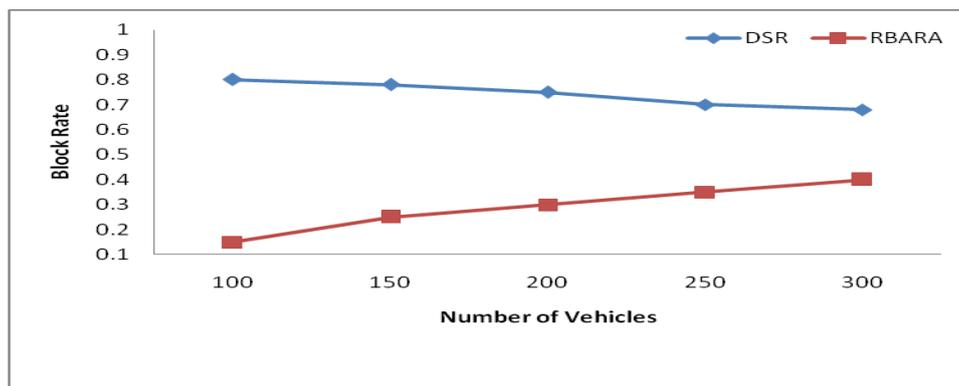
Fig. 6 Request block rate with DSR vs. Road Based Routing Algorithm in HWN
