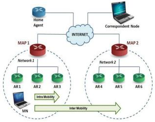
Fig2. Hierarchical Mobile IPv6 Architecture
