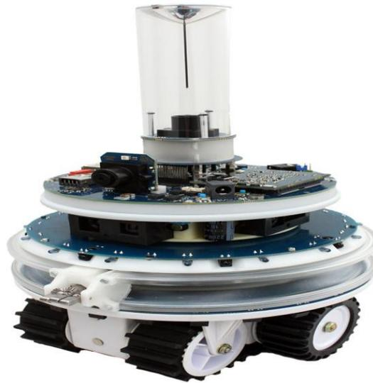
Fig. 2 Hardware implementation of hand gesture recognition system.
