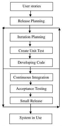
Figure 1: simple agile methods life cycle.
