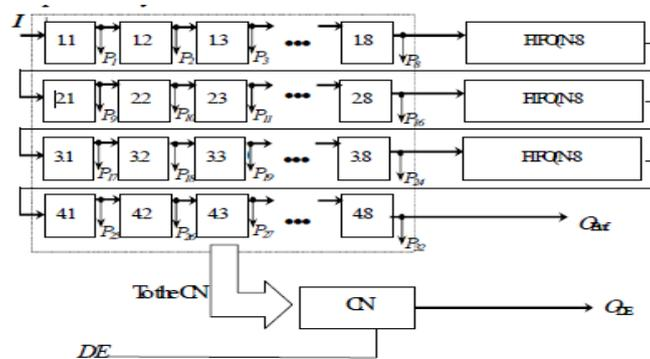
Fig 2. The FIFO array for PDEU, where the numbered rectangles represent shift registers (SR)
