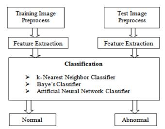
Fig.3 Block Diagram of the Proposed System
