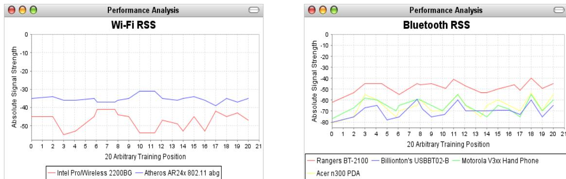
**Fig.10: Performance for Wi-Fi RSS and Bluetooth RSS**
