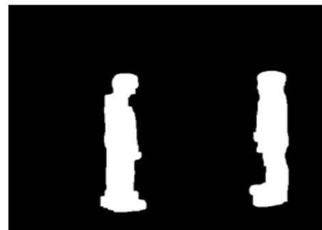
Fig.2 (b) After erosion
