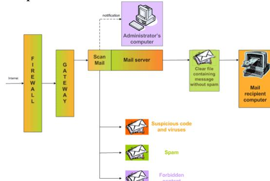
**Figure 1:** Spam Filtering Architecture
