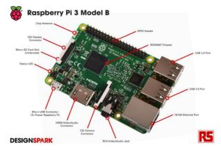
Figure 1: Raspberry Pi 3 Model B and its Features.
