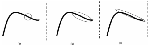
Figure 6- Curvelet with fixed orientation and location and varving scale [7]
