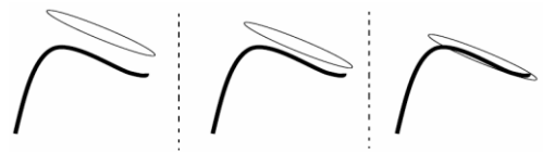
Figure 7- Curvelet with fixed orientation and scale and varving location [7]
