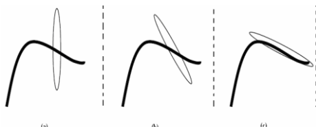
Figure 8- Curvelet with fixed scale and location and varying orientation [7]
