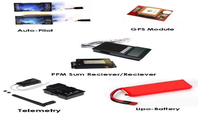
Fig.3. Flying Control and on board Equipments used in Drone
