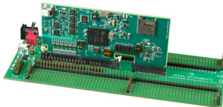
Figure 3. Texas Instruments controlCARD docking station [20]
