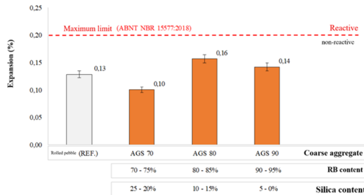
Figure 6 – Reactive potential of the coarse aggregates, obtained from the AAR (Alkali-Aggregate Reaction) analysis
