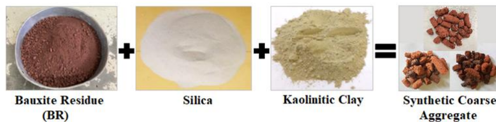
Figure 1 – Raw materials used in the composition of the synthetic coarse aggregates (adapted from 34 ).
