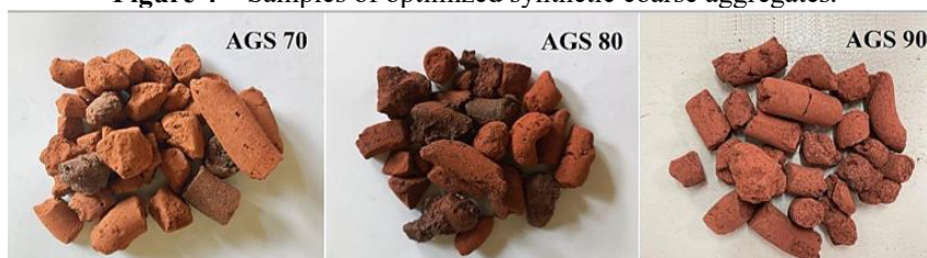
Figure 4 – Samples of optimized synthetic coarse aggregates.
