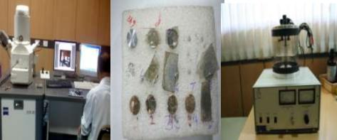
SEM Coated Stubs Carbon Coating unit Fig-5:Samples preparation for SEM and EDX analysis.
