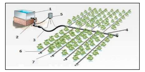
Legend: 1 - water tank 2 - control valve 3 - main line 4 - secondary line (ramp door) 5 - filter 6 - lateral line (ramp) 7 - micro-tubes (drippers)
