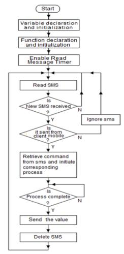
Fig.2: Flowchart of SMS Control of VI
