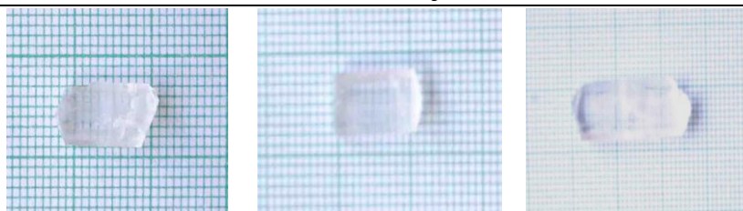
Fig 2. Photographs of the as grown (a) pure LAM, (b) La 3+ -LAM and Nd 3+ -LAM crystals
